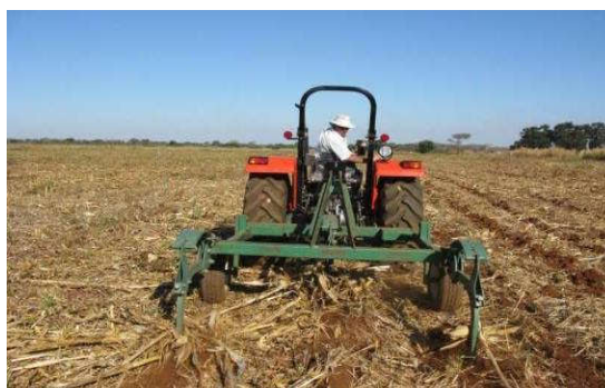
Figure 1: Mechanised Min Till (Tractor drawn ripper)
